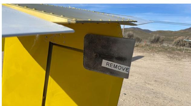
When parked, a metal rudder lock is placed at the top of the rudder and the control stick is secured with the seat belt for the ailerons and elevator.
